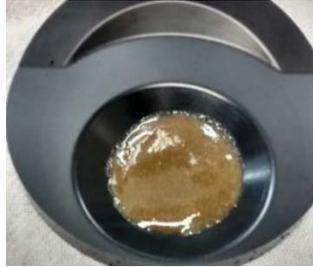
*Fig. 5 Seed magma sample in slurry cup*
